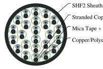
SHF2 Sheath Stranded Copper Conductor Mica Tape + HFEPR Insulation Copper/Polyester Tape + Drain Wire
